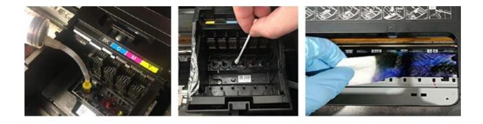
7. Allow the solution to soak for approximately 1 hour to dissolve the blockage. Repeat the cleaning process as needed for each colour.
